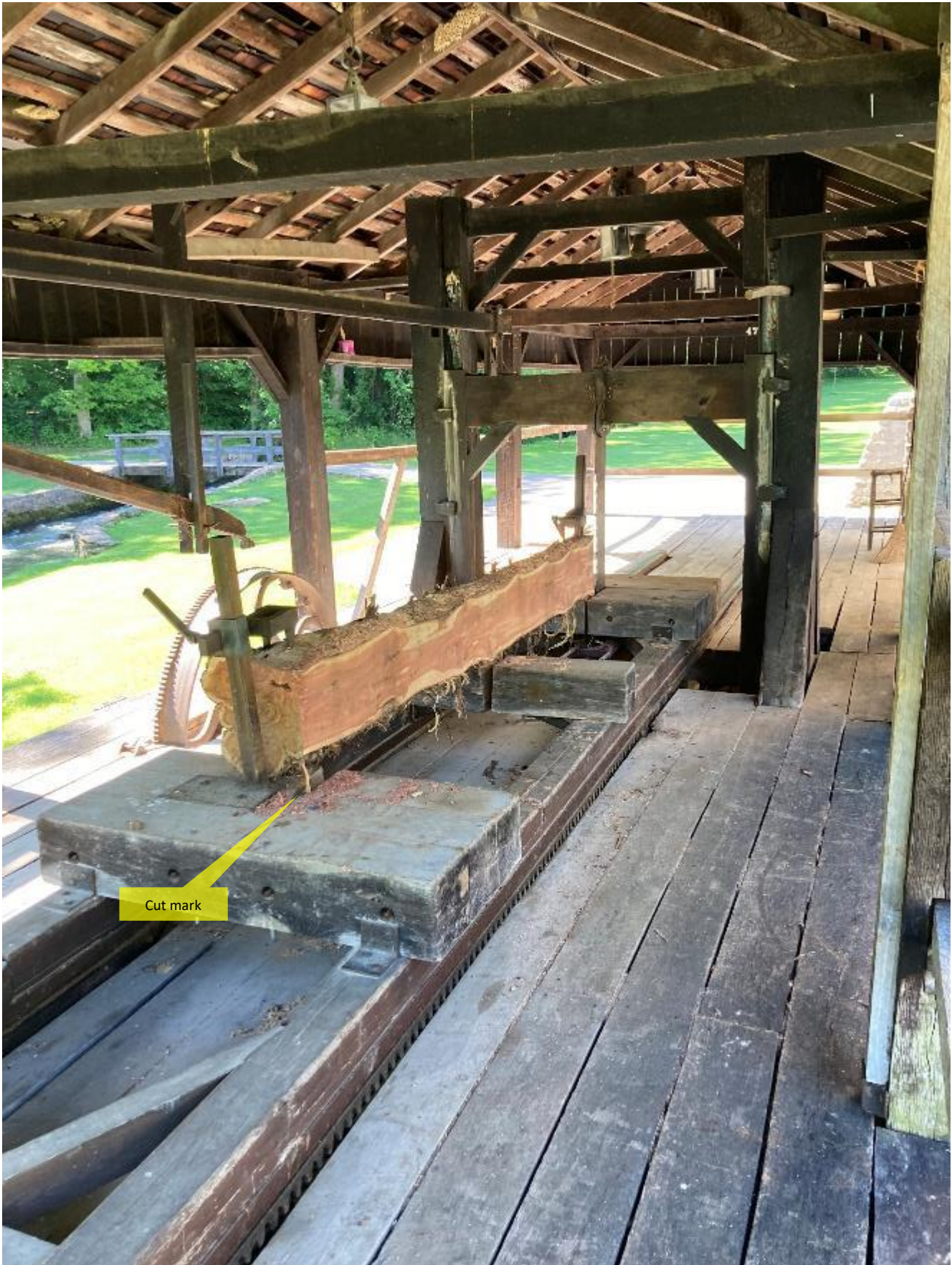
While this is an up-and-down sawmill, its reconstruction relies heavily on modern fabrications and mechanisms. The deep cut mark into the tail block denotes the lack of using a cleat to stop the saw 3 inches from the end of the log, as directed in Evans.
