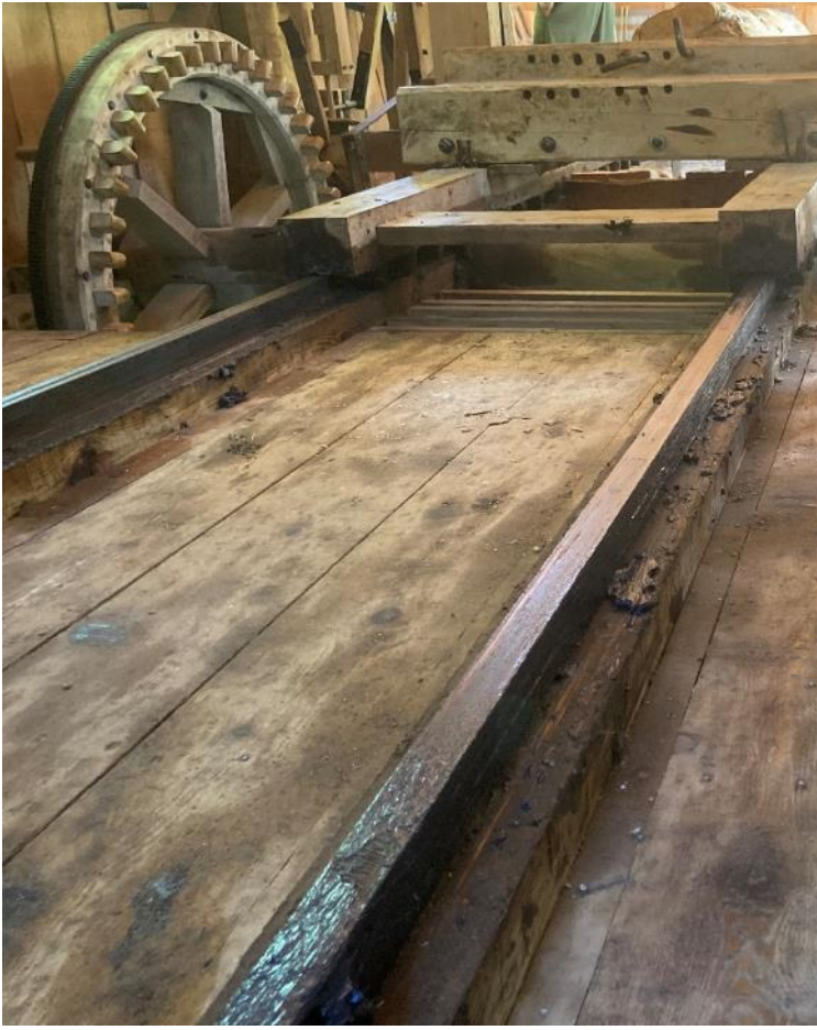
Wooden beams used as ways for the carriage. Heavily greased.
