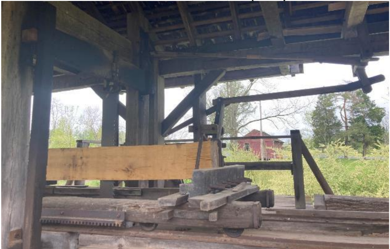
Saw frame, carriage, and associated mechanisms. Notice the post-18th century metal rails, metal carriage wheels, and toothed rails attached to the carriage
