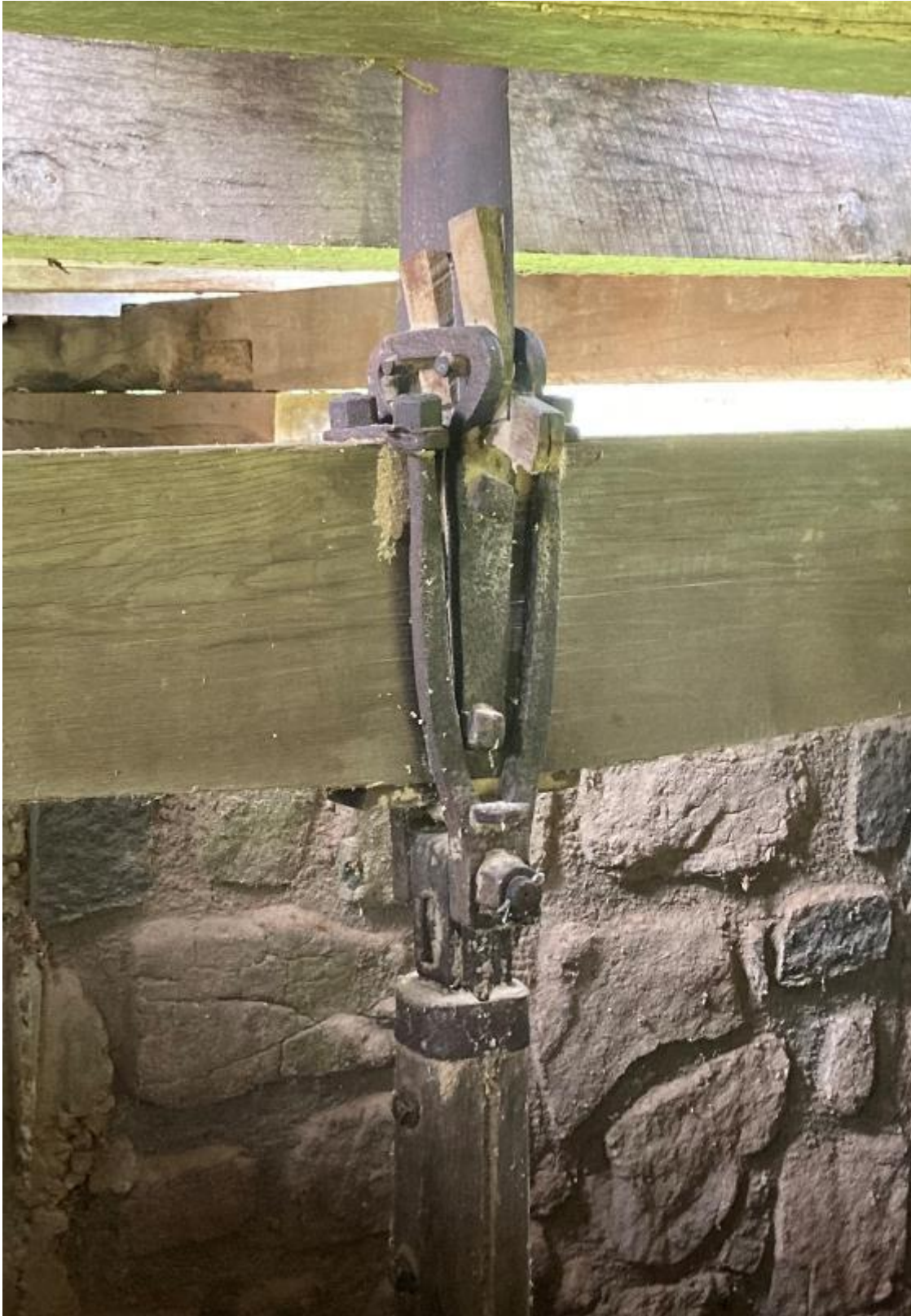
Bottom of saw blade collar attached to the pitman. Bolts to tighten saw are on either side of the blade.
