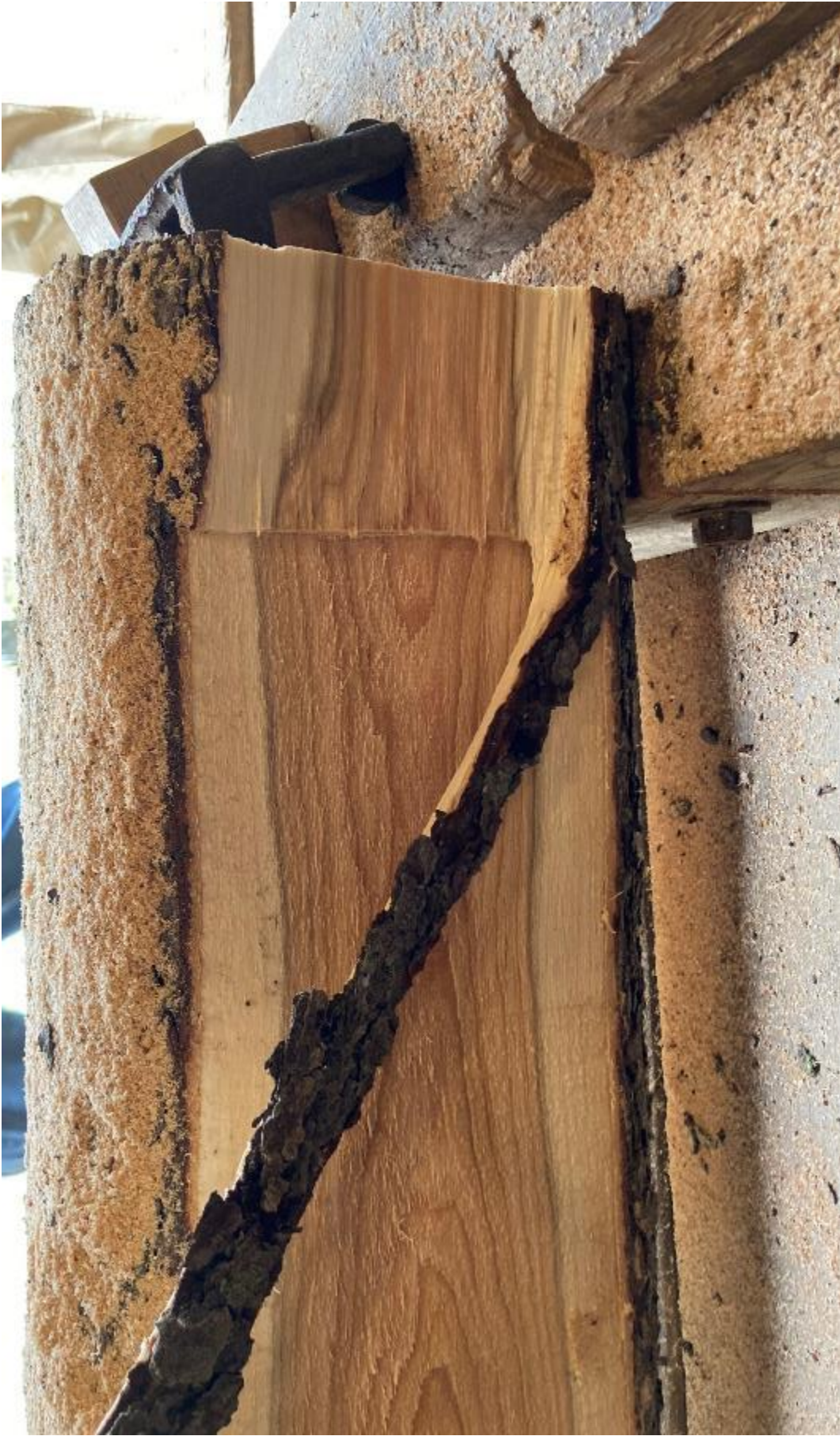
3 inches of uncut wood, indicative of the use of a cleat to stop the sawing momentum, as detailed in Evans's The Young Mill-Wright .
