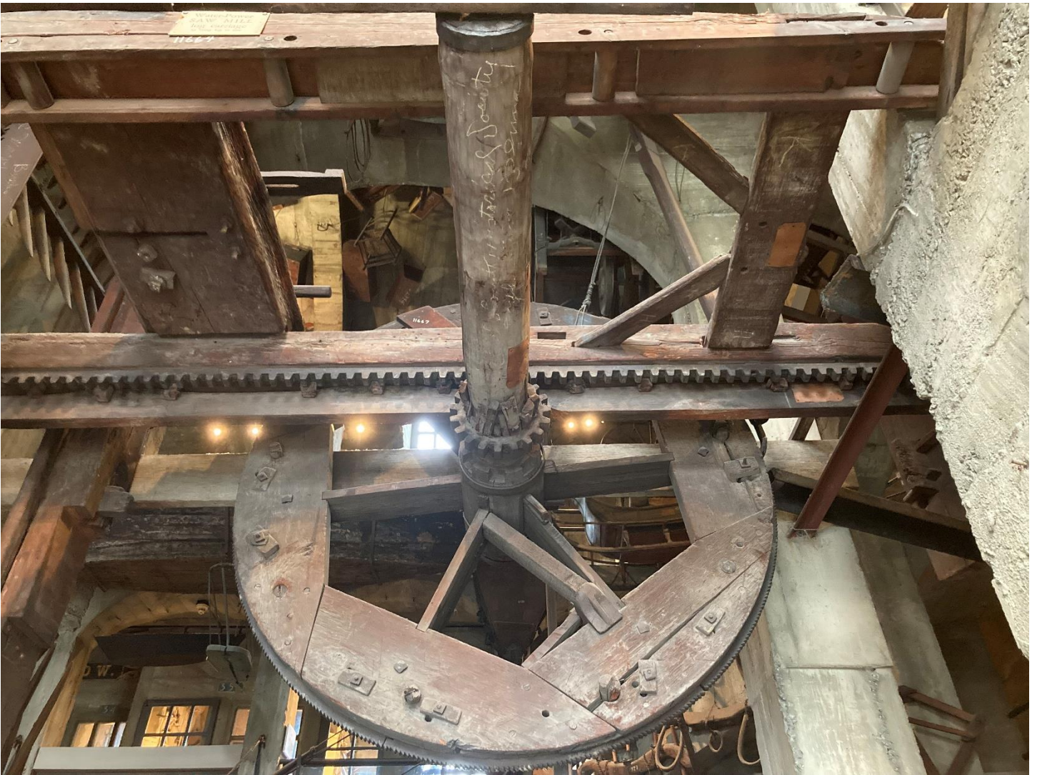
This picture shows parts of a sawmill in the Mercer Museum. This way of propelling the carriage utilized metal gearing, which was common in 19th century sawmills. This type of gearing is what moves the reproduction sawmills at Old Sturbridge Village, the Bertolet Sawmill, and the Spring Mill Sawmill.
