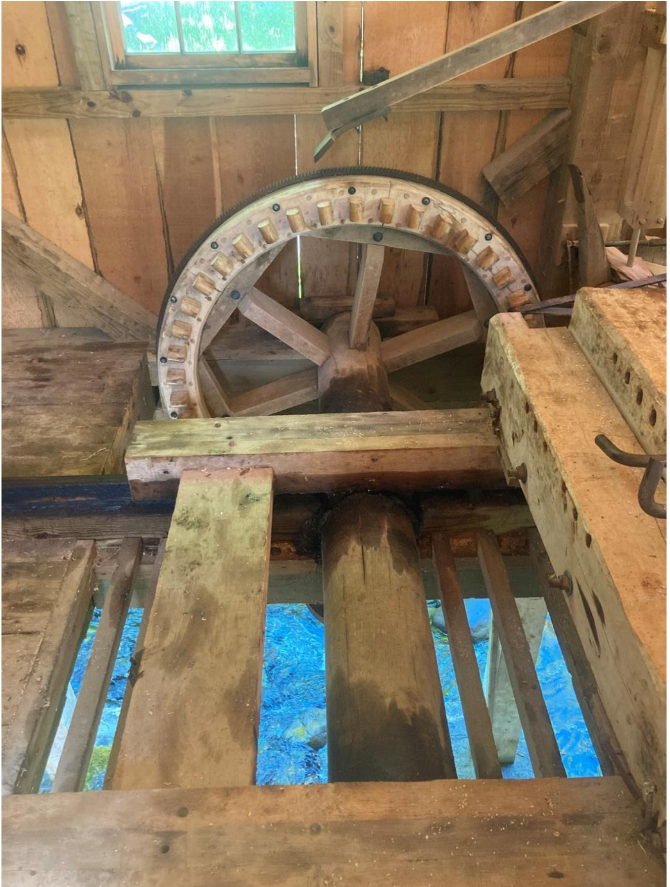
Rag wheel that moves carriage forward and backward.
