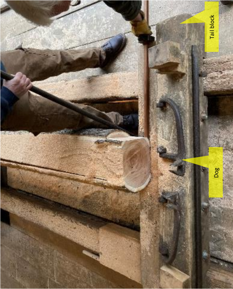
Volunteer uses an iron bar to move the log over, using precise measurements to gauge the thickness of the cut.
