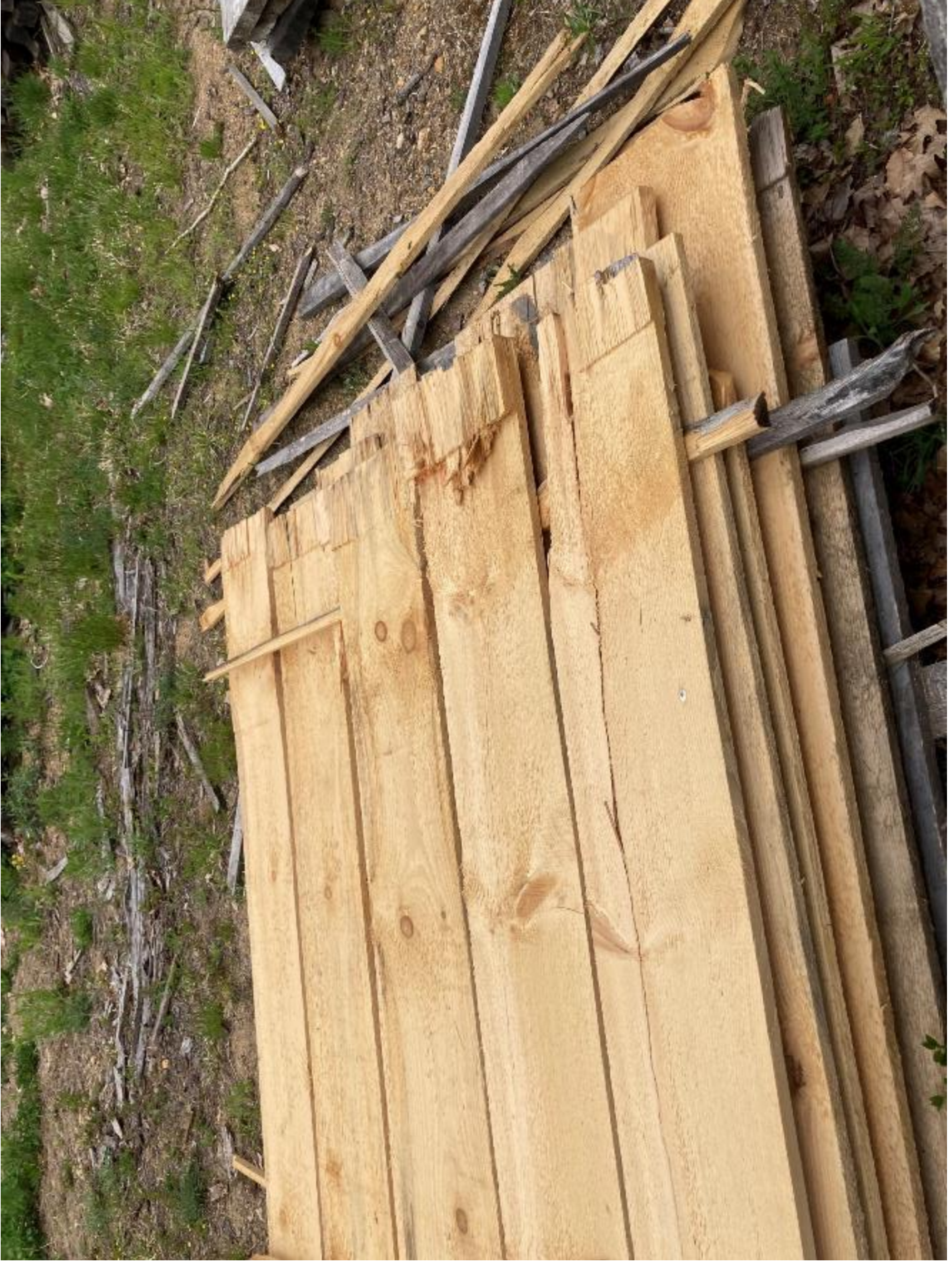
Stacked, sawn lumber. Notice the 3 inch unfinished marks of the ends, indicative of proper sawing techniques. Carpenters could remove these marks by using a plane to level the lumber, cut the end off, or use the lumber as is.
