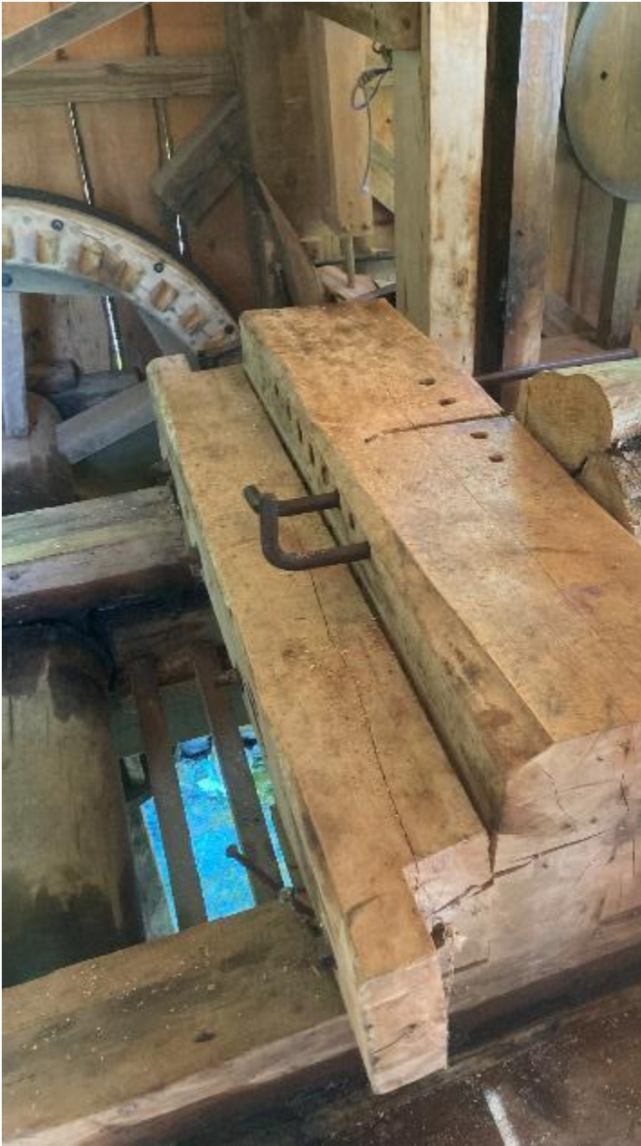
Simple dogs that drive through holes in the head and tail blocks directly into the timber. There should be dogs also holding the top of the timber. Without these, the log may bounce from sawing, causing damage to the carriage, the ways, and saw blade.
