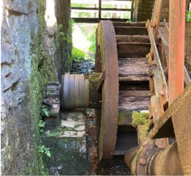
Flutter wheel under the sawmill.
