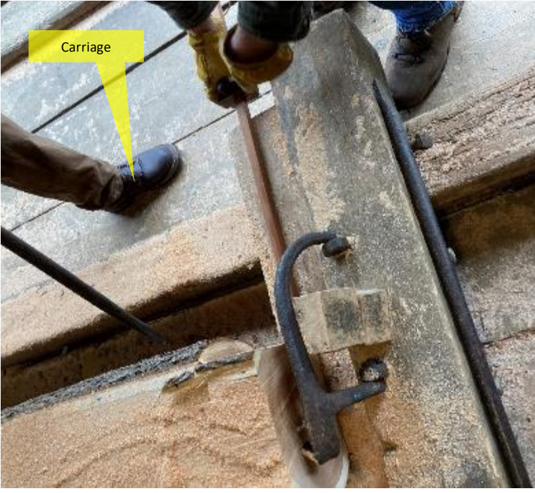
Volunteer uses an iron bar to move the log over, using precise measurements to gauge the thickness of the cut.
