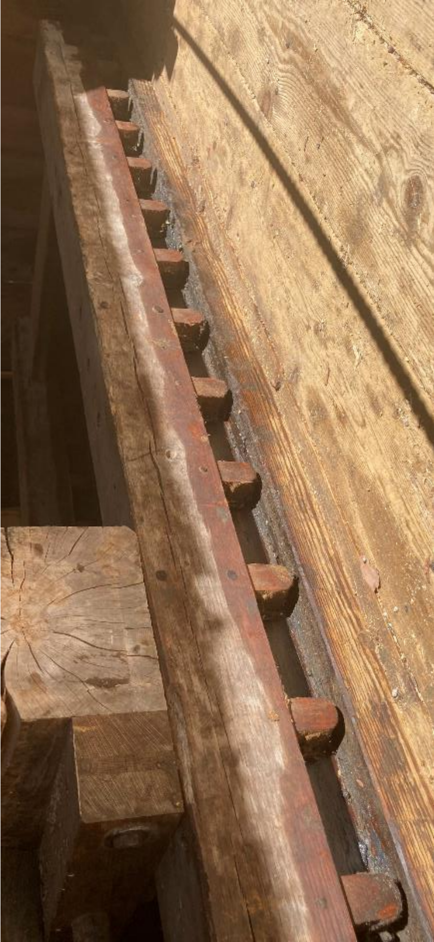
Wooden cogs mounted to both sides of each side of the carriage frame. The cogs keep the carriage on the ways.
